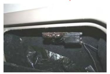
**Trunk Latch used to Lock Compartment**
