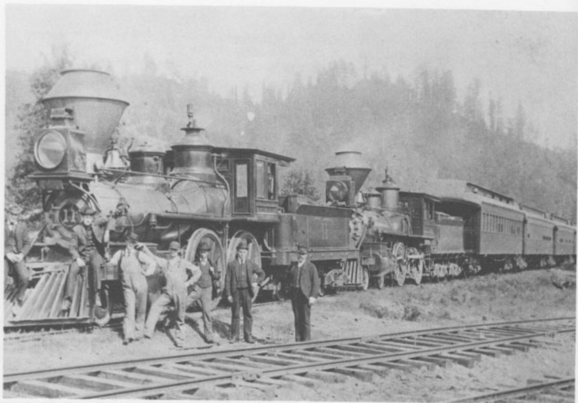
Diamond stack woodburners, Nos. 11 and 10, of the SF&NPRy., with the first train to Camp Vacation. (W. A. Silverthorn Collection.)
